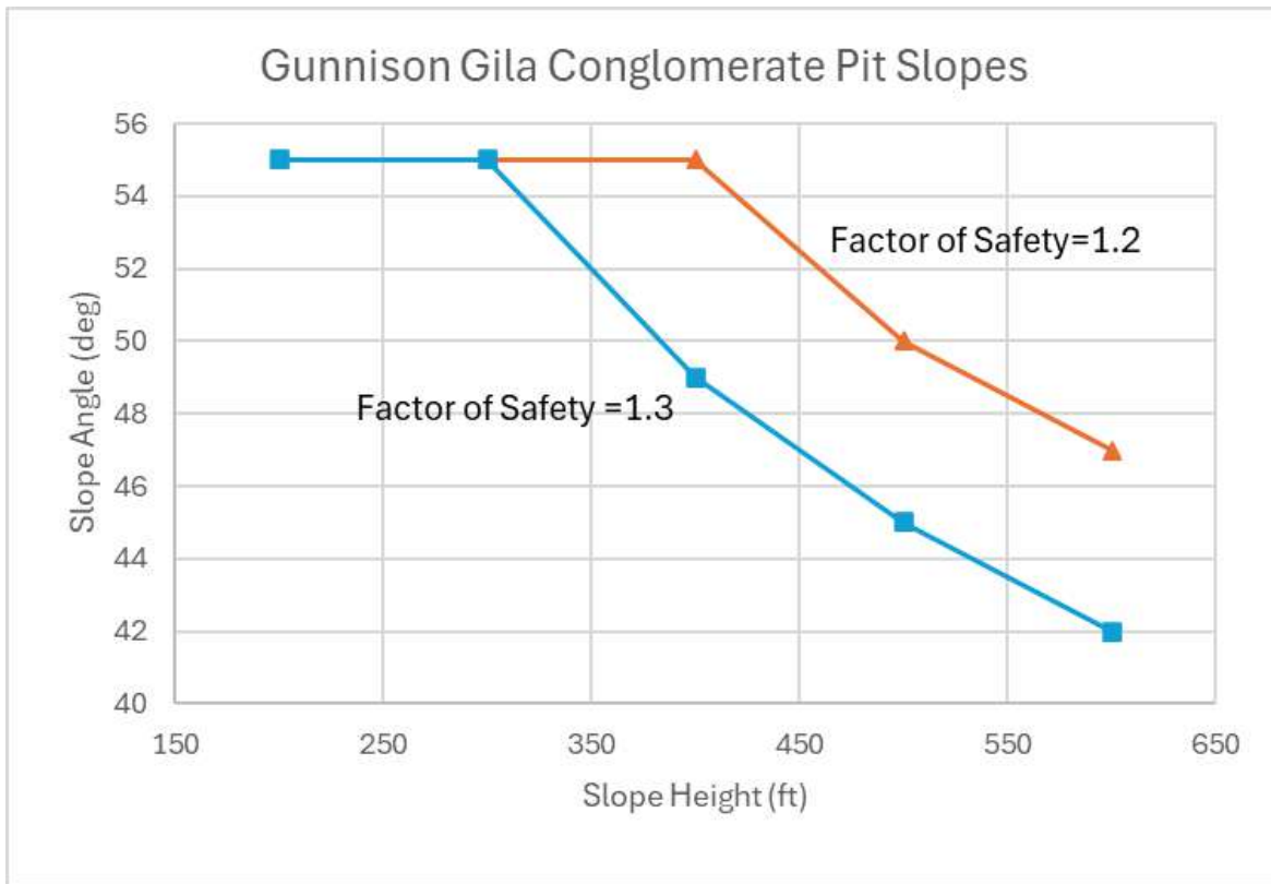
Figure 16-5: Gila Conglomerate Slope Height versus Slope Angle for Factors of Safety of 1.2 and 1.3
